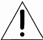
The exclamation point within an equilateral triangle is intended to alert the user of the presence of important operating and maintenance (servicing) instructions in the literature accompanying the appliance.
